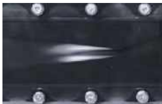
CAVITATION IN THE VENTURI
