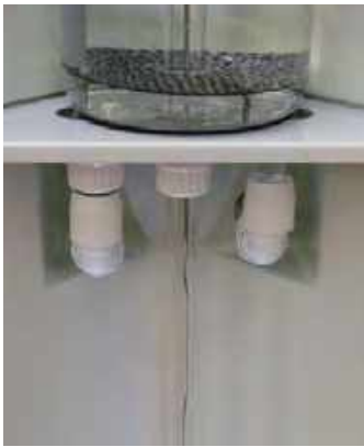
DYE STREAM SHOWING LAMINAR FLOW
