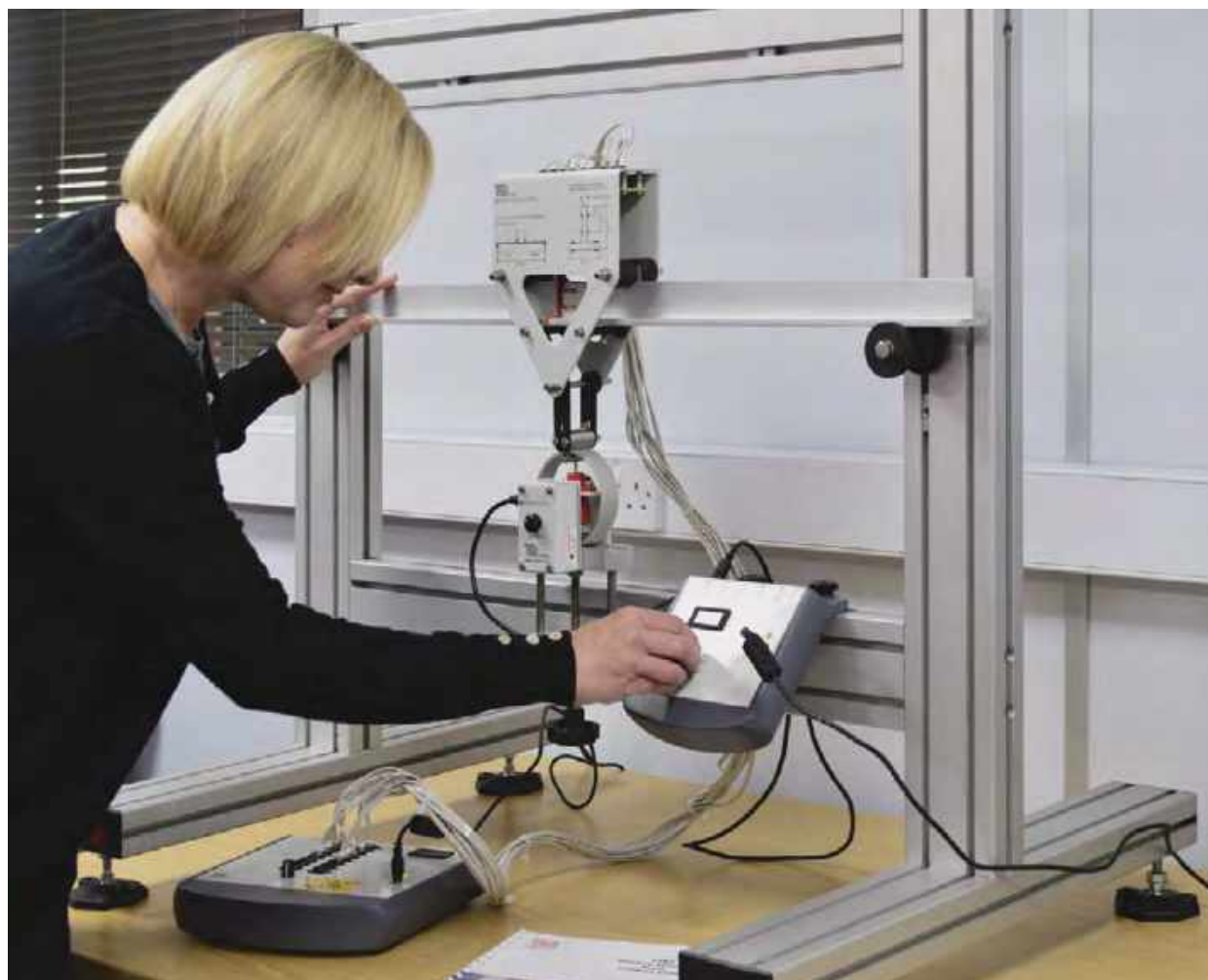
TEST FRAME (STR1) FITTED WITH THE EXPERIMENT MODULE BENDING STRESS IN A BEAM (STR5) AND DIGITAL FORCE DISPLAY (STRIA)
