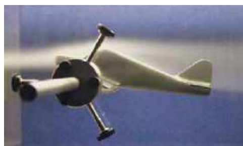
SMOKE TRAIL AROUND THE LOW WING AIRCRAFT MODEL
